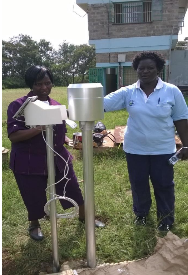
From Left, Manual Rainfall Station Versus, Right, a Modern Rain Recorder.
